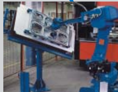
2. At the orientation table the workpiece is automatically positioned before bending.
