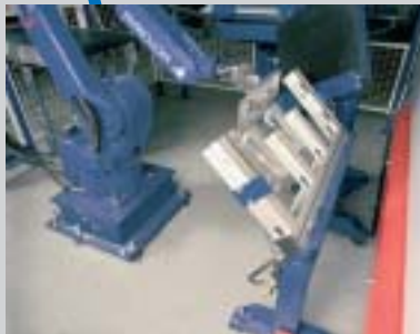
4. The regrip station, in front of the press, is used when the robot needs to change its grip between different bends.
