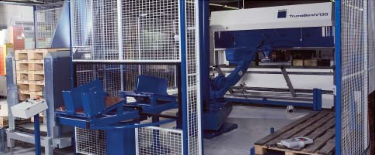
The rotating sheet magazine has two stations and can be loaded while the cell is in operation.
