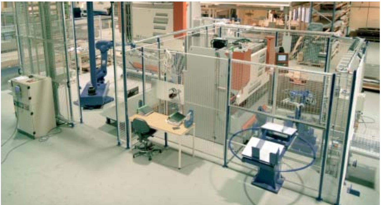
Motoman's turnkey system with robotised press-brake operation. The turnkey systems have different options for collecting sheets and placing the finished products on pallet or roller conveyor.
